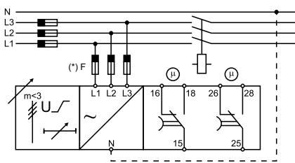
Connect the 3-phase power supply and the neutral (if present) taking care of the sequence. Connect the relay output according to the ratings.
