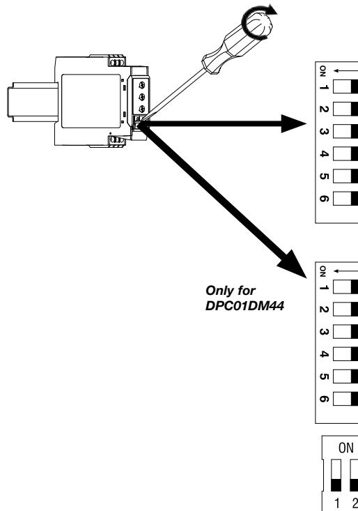
To access the DIP switches open the plastic cover using a screwdriver as shown on the left.
