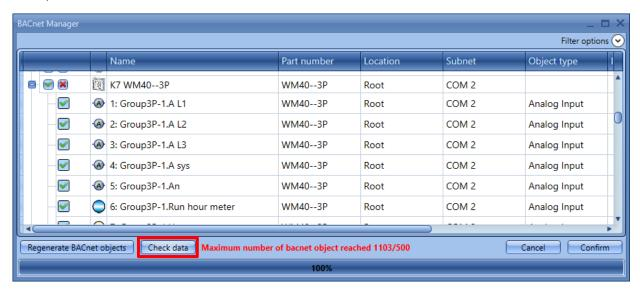
As shown in the example above, a warning message will be displayed if the maximum number of BACnet Objects has been exceeded and their amount; otherwise the *Ok* message will be displayed when it is compliant.
